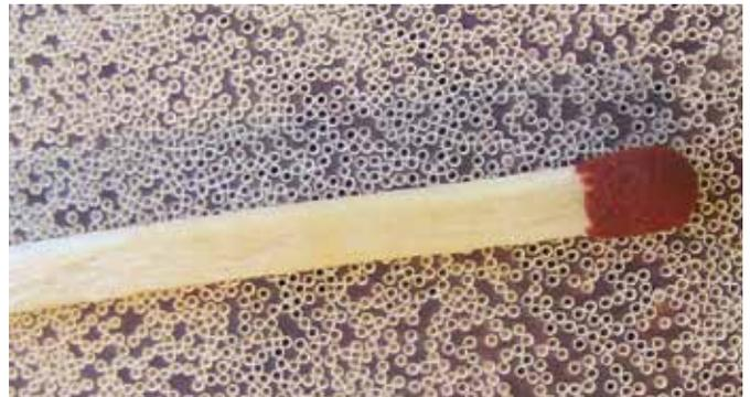
Parker has other useful technologies for gas treatment – generally developed for compressed air. These include drying (dew point suppression) using membrane technology (see catalogue S3.2.111), and membrane gas separation of air into nitrogen and oxygen. (see catalogue K3.1.075)
