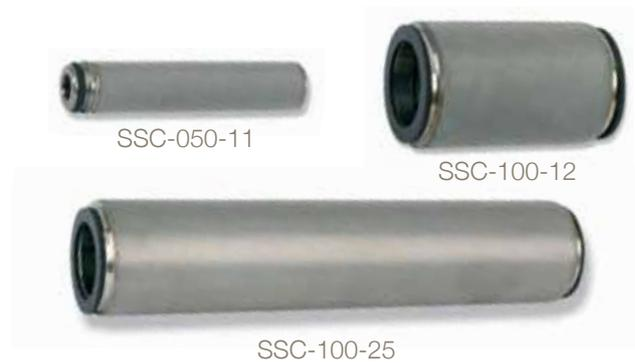
Three standard efficiency ratings from 1.5 to 15 microns nominal, 5 to 25 microns absolute (others available) and three standard sizes are available. SSC cartridges are re-usable and may be cleaned using back flushing, chemical or ultrasonic methods. Therefore they are especially suited to applications
